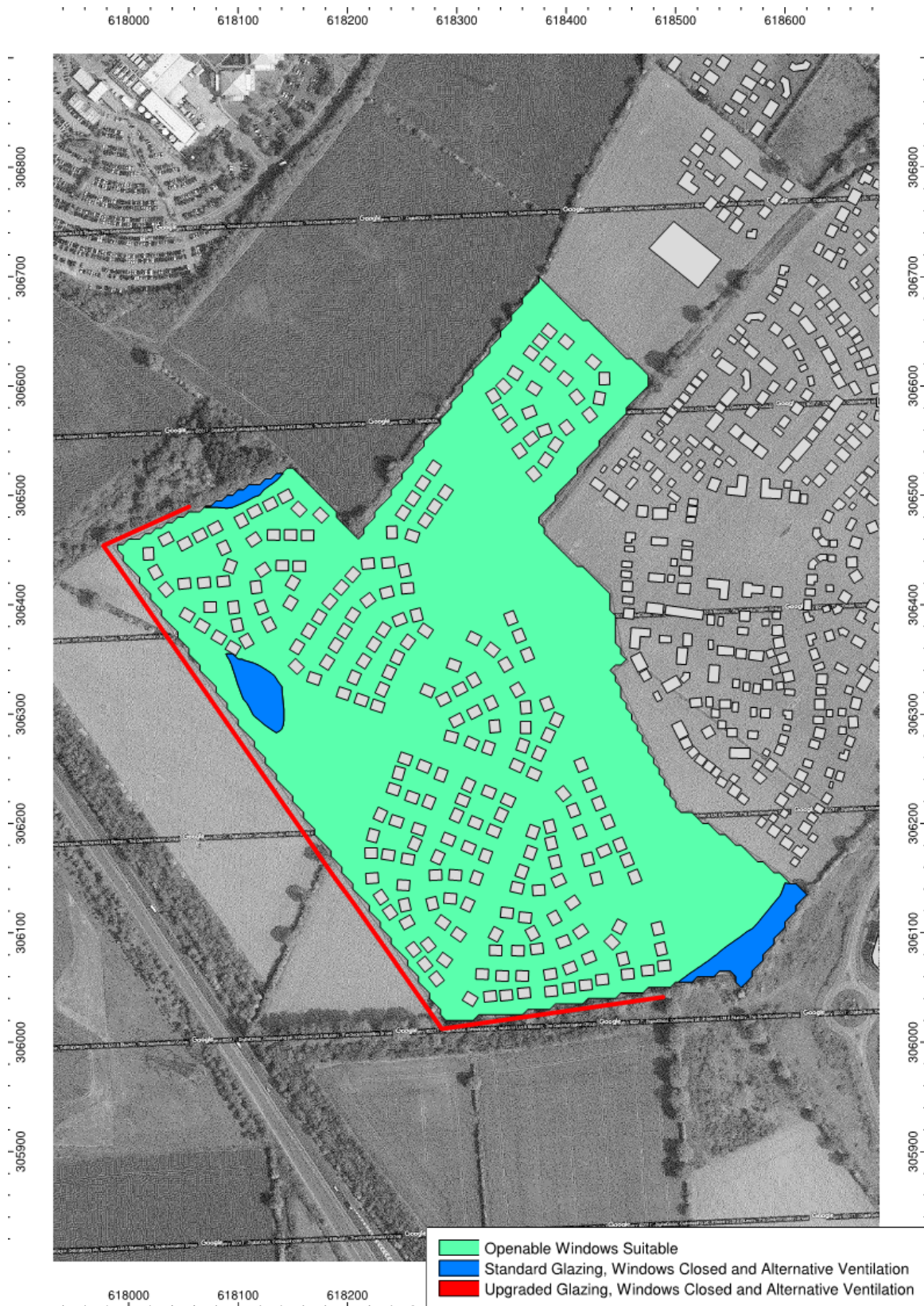
Figure 7: Night-time BS8233 Internal Amenity Constraints (First Floor) – Mitigated site using 8 metre barrier
