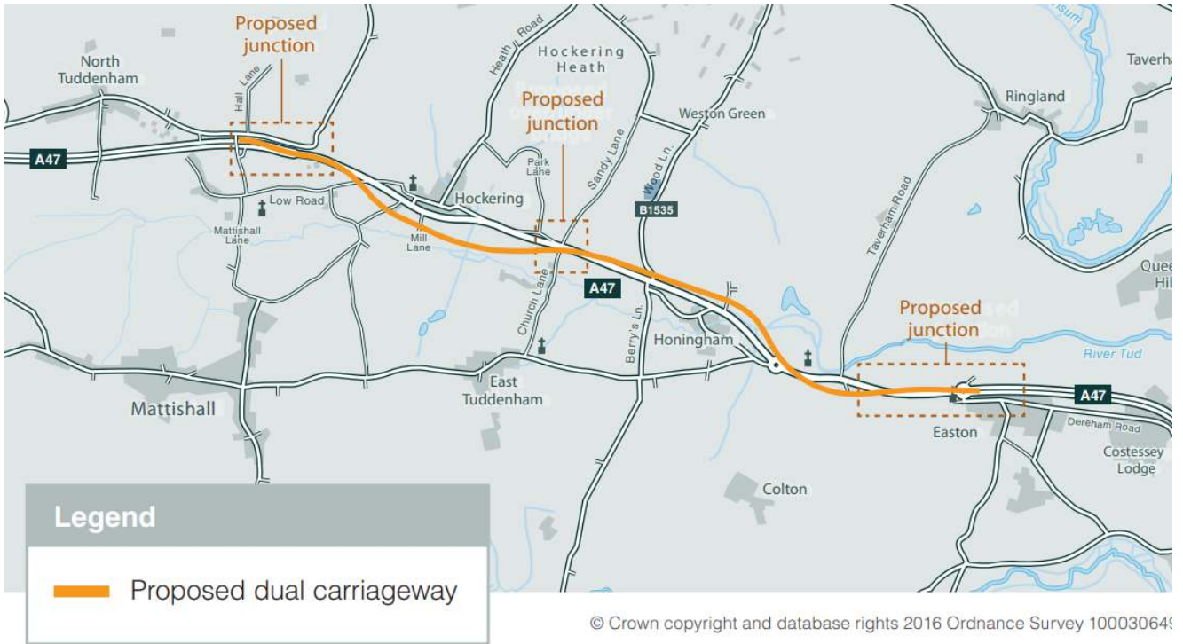
Proposed A47 North Tuddenham to Easton Dualling (for full scale map see NCC Website)
